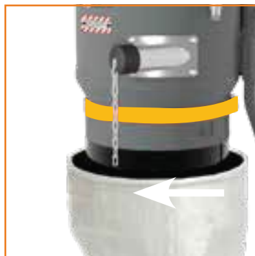
8. Bring the inside of the bag up to the height of the belt positioning. Close the bag around the chamber with the belt.
