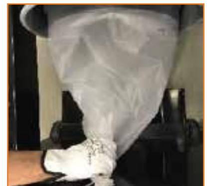
9. Pull the bag and place at the edge the band to create a new one. If necessary use two bands.
