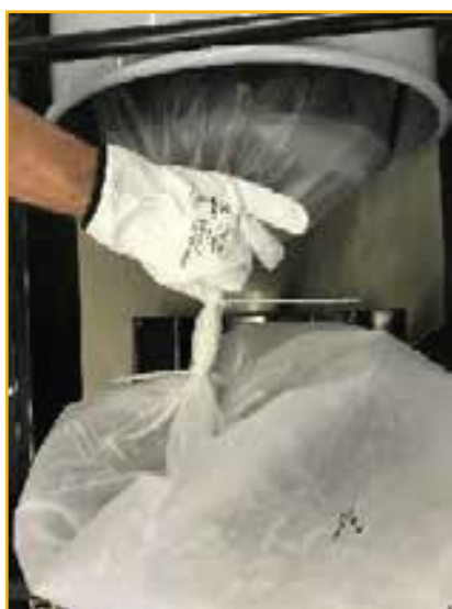
1. Close the bag with two distanced bands.
