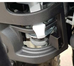
Fig4: Warm start or trouble start position - Engine Fuel tap lever (black) to the right and choke lever (grey) in centre position. Don't forget to move this choke lever immediately to the right (off position) when the engine starts running
